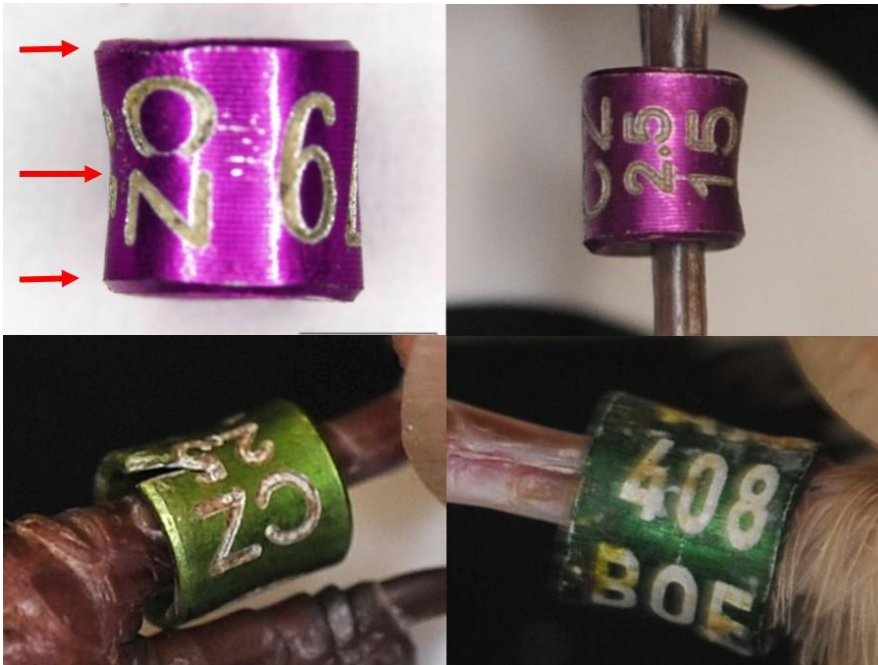
Rings with concave shape (Top left: Heidenblut Institute for Materials Science at the University of Hanover. Others: Cologne Public Prosecutor's Office)
