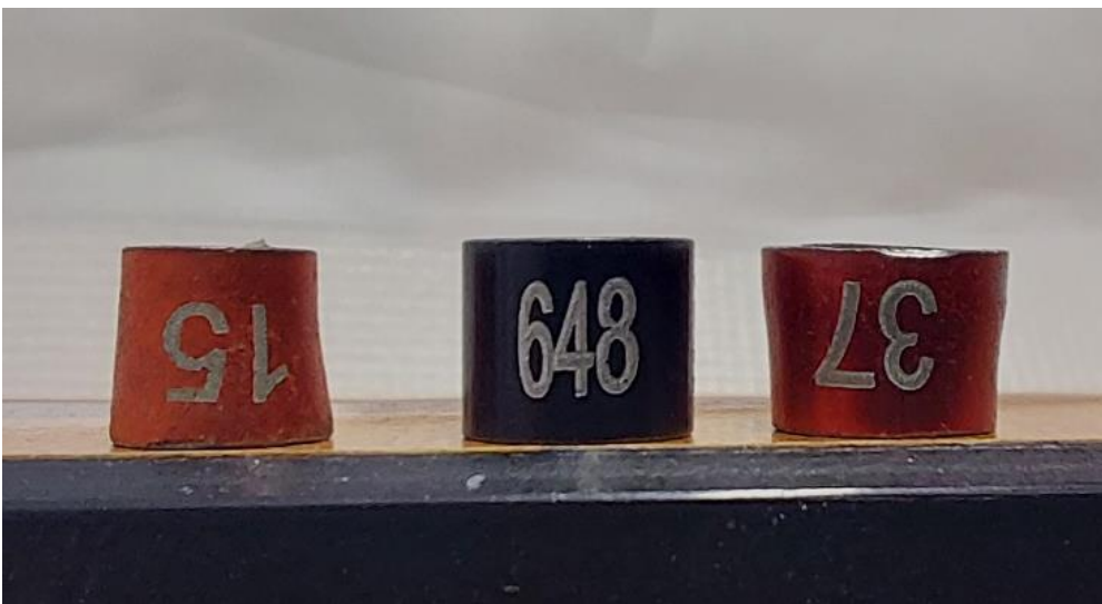
Manipulated rings on both sides and non manipulated ring in the middle (E. De Santis)
