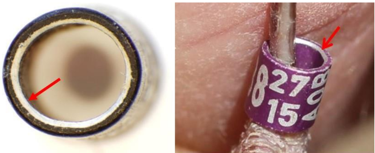
Rings with beveled inner edge (Left: Heidenblut Institute for Materials Science University of Hanover. Right: City of Cologne).
