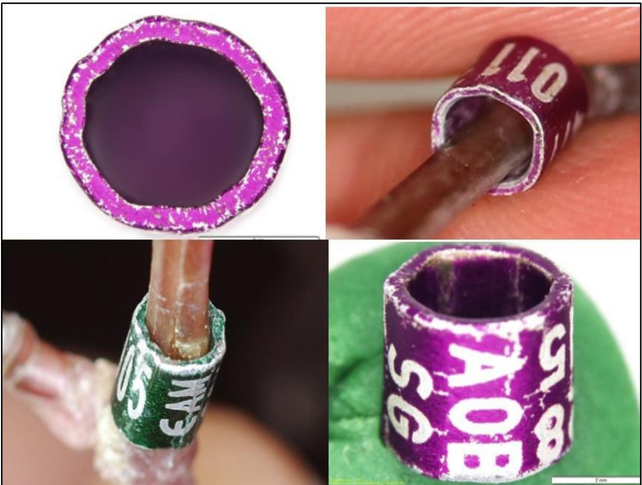
Rings with a wavy edge (Top left and bottom right: Heidenblut Institute for Materials Science at the University of Hanover. Others: City of Cologne).
